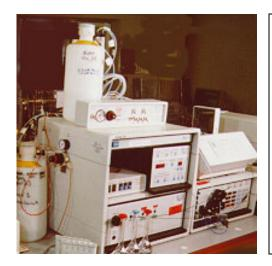
The ion chromatography is used for the analysis of aqueous samples in parts-permillion (ppm) quantities of common anions such as fluoride, chloride, nitrite, nitrate, and sulfate and common cations like lithium, sodium, ammonium, and potassium using conductivity detectors. The chromatography also has the capability to analyze aqueous samples for parts-per-billion (ppb) quantities of hydrazine, monomethylhydrazine (MMH), and unsymmetrical dimethylhydrazine (UDMH).
