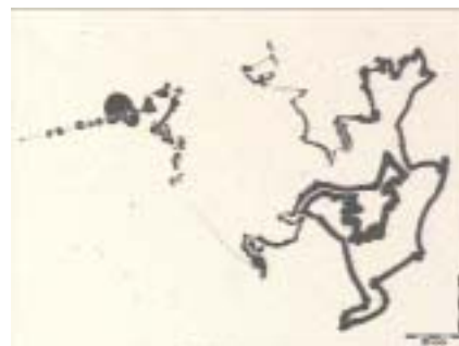
Fig. 2 Filiform corrosion on a corroded compact disc (100X)
