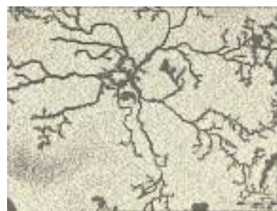
Fig. 3 Simulated filiform corrosion on compact
