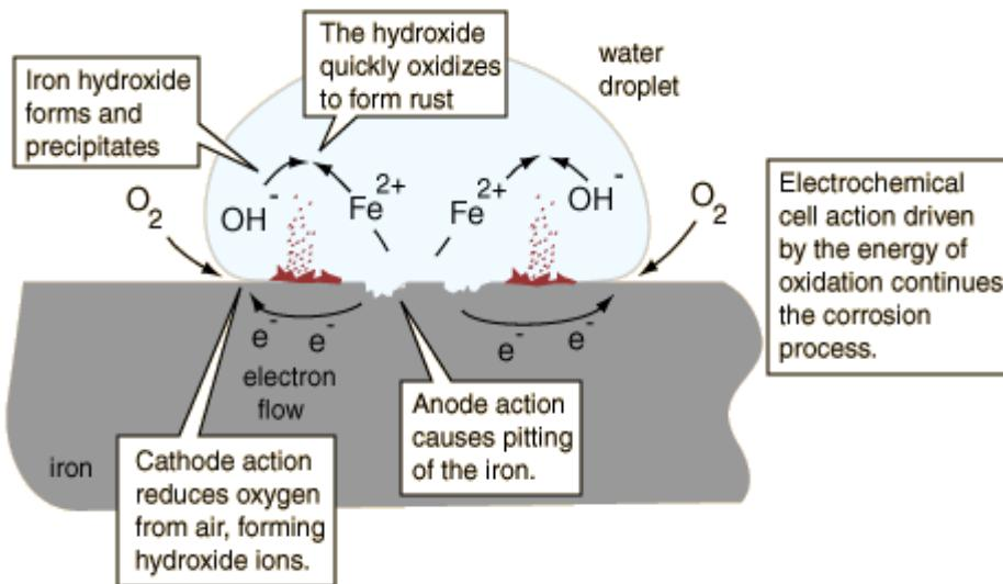
7. A piece of bare iron left outside where it is exposed to moisture will rust quickly. The corrosion rate is enhanced by an electrochemical process in which a water droplet becomes a voltaic cell in contact with metal, oxidizing the iron.
