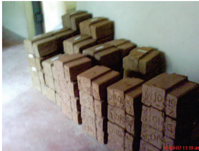
Figure 2. Stacking of Lateritic Interlocking Blocks
