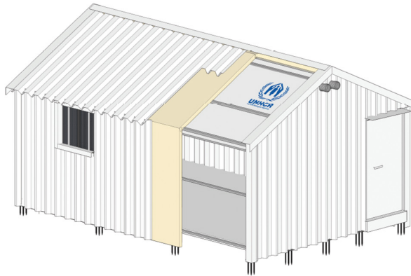
Figure 1. T-shelter cladded by aluminium foam insulation between two IBR sheets Source: UNHCR (2015)
