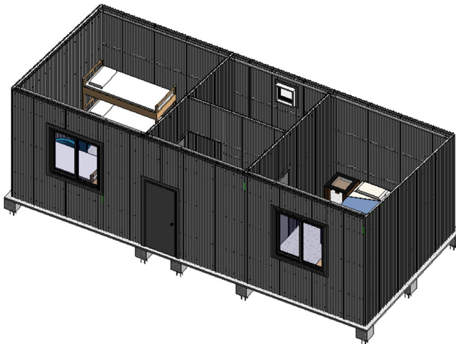
Figure 11. IBR cladding the structural steel frame
