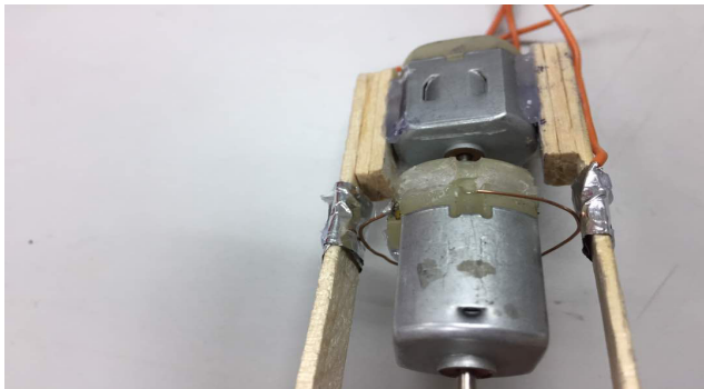
Figure 5: The aluminium foil and the extended copper wire that allows voltage flow out from the generator.
