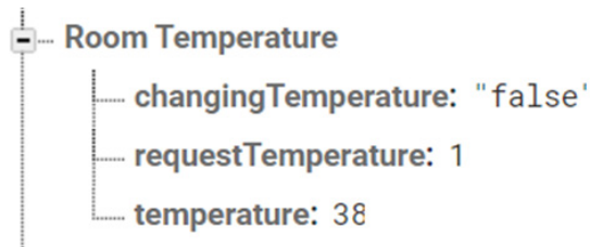
Figure 26: Changes in requestTemperature to Request Turning OFF Air-Conditioner
