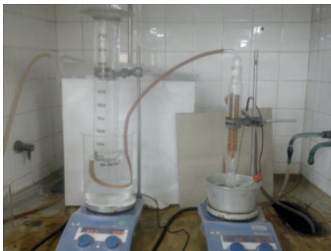
Figure 1: The reaction set up (on the right) and the arrangement for the downward displaced collection of the hydrogen gas (left measuring cylinder).
