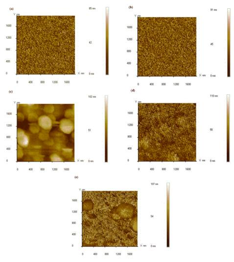
Figure 1: AFM images of bimetallic chips (a) silanised with APTES by (b) APD, (c) OPD, (d) CVPD and (e) DVPD methods.
