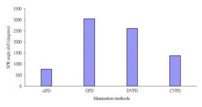
Figure 3: Amine accessibility for various silanisation methods.
