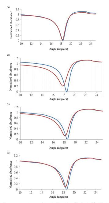
Figure 2: SPR response of sputtered thin Au/Ag films silanised with APTES by (a) APD, (b) OPD, (c) CVPD and (d) DVPD methods.
