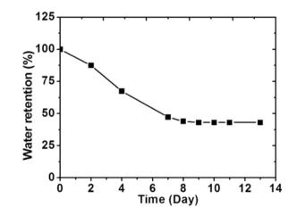
Figure 5: Effect of standing time of SAP on water retention (CMC/AAc = 1.0:1.5, room temperature =  $27^{\circ}$ C, dose = 5 kGy).
