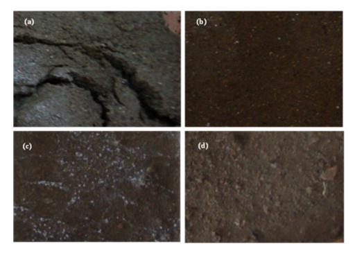
Figure 8: Photos of (a) the soil without SAP, (b) the soil with 0.1 wt% SAP, (c) the soil with 0.2 wt% SAP and (d) the soil with 0.4 wt% SAP.
