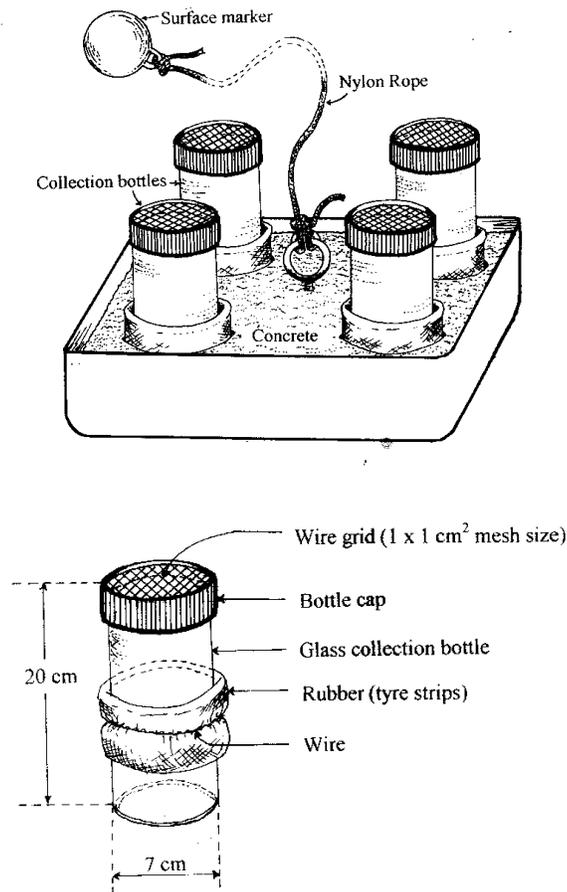
Figure 2: Sediment trap
